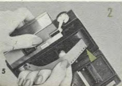
2. Pull down rewind lever (on camera bottom) and turn film take-up drum until metal hook is on top. Push rewind lever back up. Place film leader over drum so one of the perforations on end engages hook. Keeping tension on film, move wind lever through a **FULL** stroke, then press shutter release.
