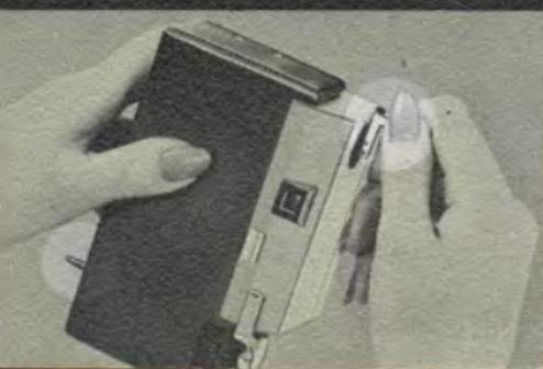
**unloading . . .** *Before camera is opened, film must be rewound.* Pull rewind lever down, release rewind crank by sliding grey button away from arrow, and rewind film until counter stops turning. Open back and pull rewind crank up to remove film.
